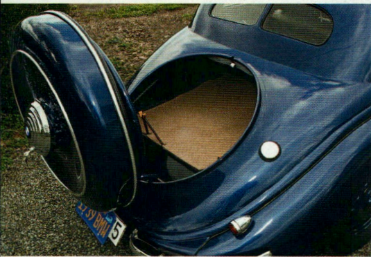
With its clean lines and flowing sheet metal, the Pillarless Coupe is a fine example of the coach-builder's art, created in Darmstadt by Autenrieth Karosserie. The spare tire holder is also the trunk lid, a clever touch. The clock and instruments are original, but the radio has been replaced.
